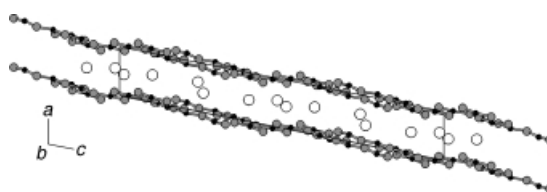
Figure 11. Crystal structure of K 3 [C 6 N 9 ], view along [010] (K + : open circles, C: black circles, N: gray circles).
